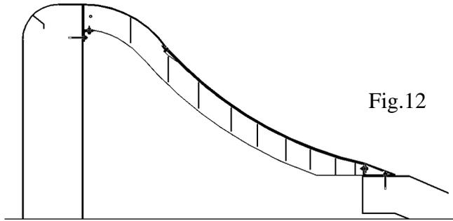
Some intake sites have large boulders in the water during floods. The intakes designed for these locations use thicker metal for the construction, heavier screens, and bars welded to the top of the screens (as well as other features).
